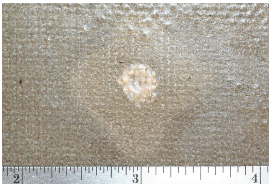
FIGURE 1 The impact to the glass fiber reinforced polyester caused noticeable deformation around the impact site, as shown in this photograph. Scale is in inches.
