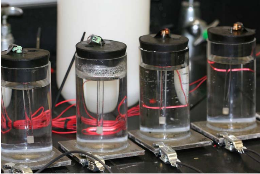
FIGURE 2 The cathodic disbondment cells are shown in the photo, attached to the composite plates via silicone adhesive.
