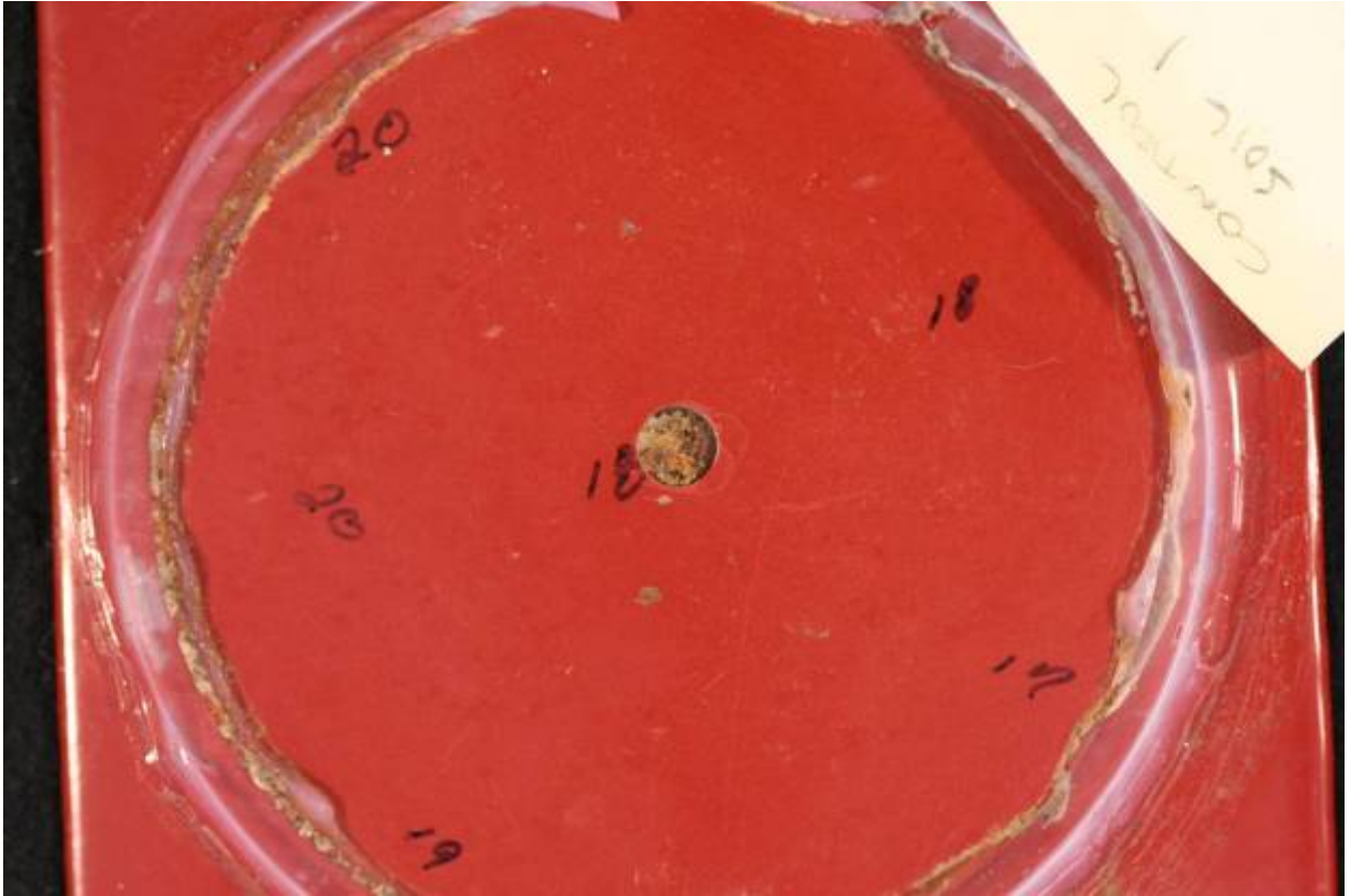
Figure 1. Appearance of the test sample (coating thickness ranges from 17 to 20 mils).
